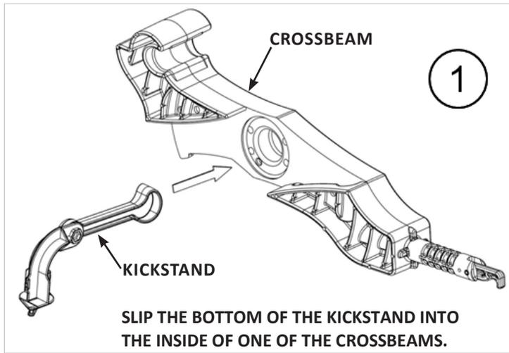
SLIP THE BOTTOM OF THE KICKSTAND INTO THE INSIDE OF ONE OF THE CROSSBEAMS.
